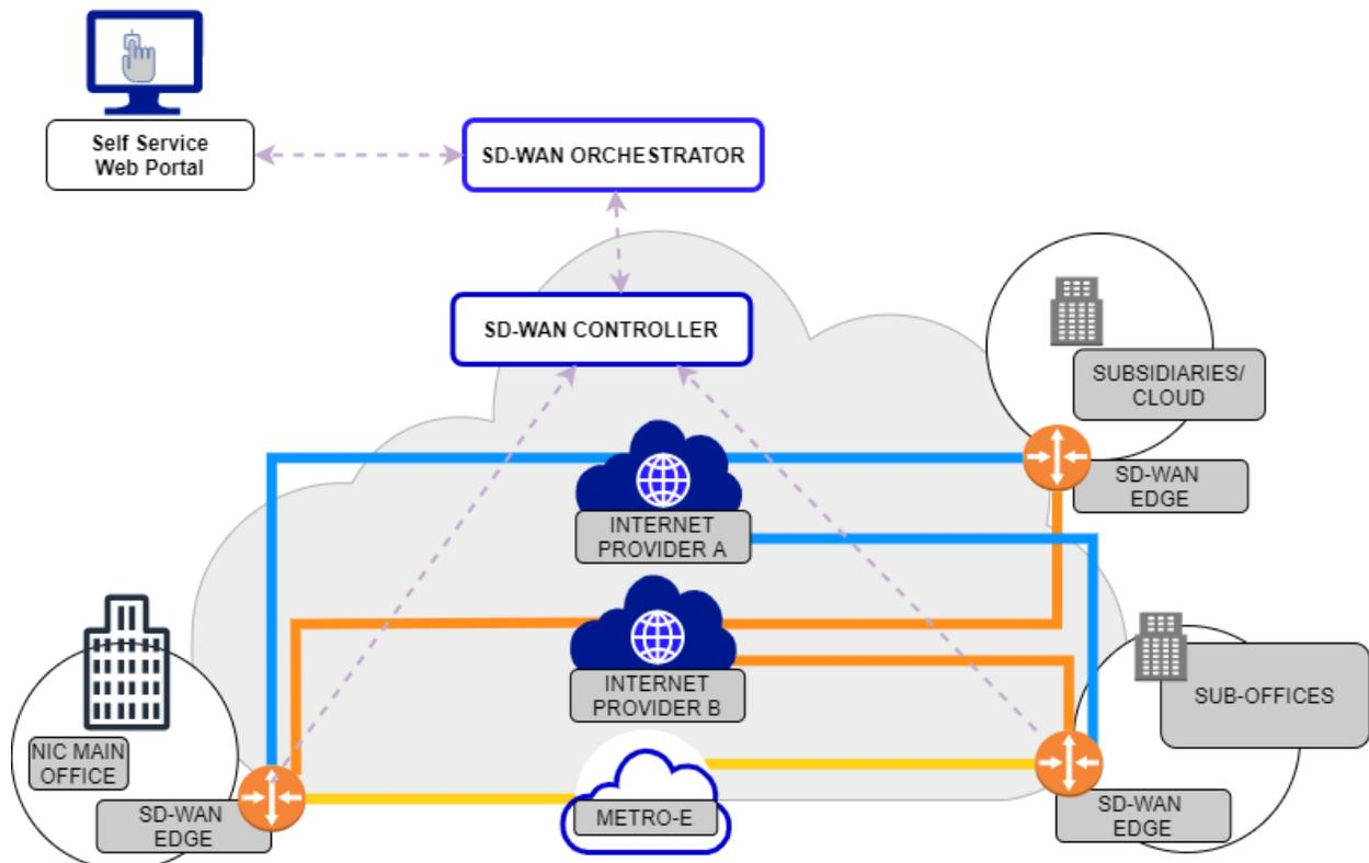
Fig 4: High-Level SD-WAN Architecture of Required SD-WAN (Thick colored lines represent SDWAN tunnel virtual connection(TVC))
