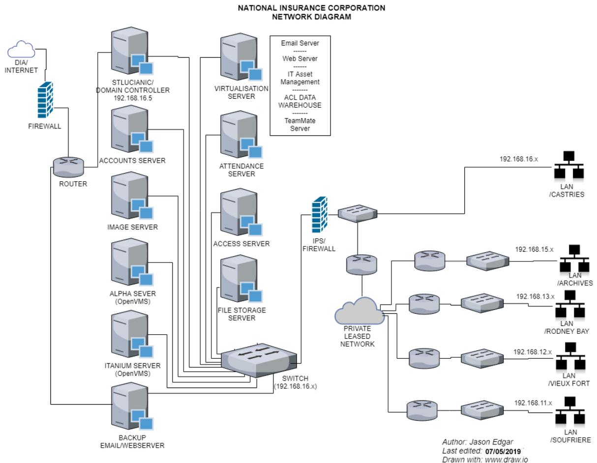
*Fig 1: Existing Network Architecture*
